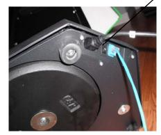
**Turning on the kiosk** – There is a complete system power switch located on the rear bottom of the base. If PC fails to turn on, see next step.
