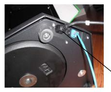
Connecting Power and Network Cables – Connect the female end of the power cord into socket located at the rear bottom of the base. Plug the male end of the power cord into a standard grounded electrical outlet. A standard RJ-45 network connection is also located on the rear bottom of the base.
