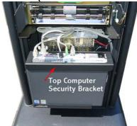
Accessing the PC —remove rear door with keys provided with the kiosk . Slide top security bracket upwards to access USB ports on PC. Turn on PC by pressing power button.
