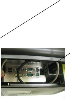
Turning on your kiosk, cont. – Inside the rear access panel, located near the power plug, there is a toggle switch for the computer. Hold for 4 seconds to force PC to shutdown. Toggle momentarily to restart.
