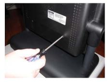
Installing software (via network or USB) Open the access panel – The system's access panel is located at the bottom of the back of the computer's enclosure. The panel is secured with two screws, either standard Philips or secure Allen screws. Remove both screws and the access panel door will swing down and out. Inside you'll see the network and USB ports.
