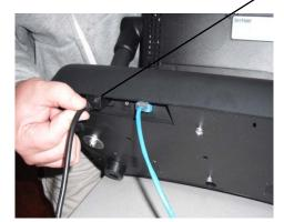
**Turning on the kiosk** – There is a complete system power switch located on the rear bottom of the base. If PC fails to turn on, see next step.
